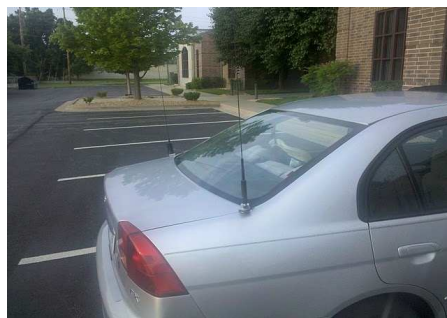
Picture of antennas installed on the Honda
