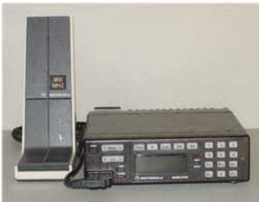
900 MHz Motorola Spectra with DTMF keypad on control head (shown with base station microphone)
