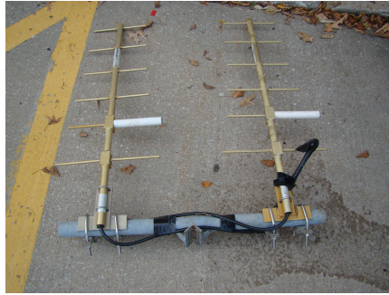
Dual UHF Yagi mount for the 53.270 Milo remote receiver site
